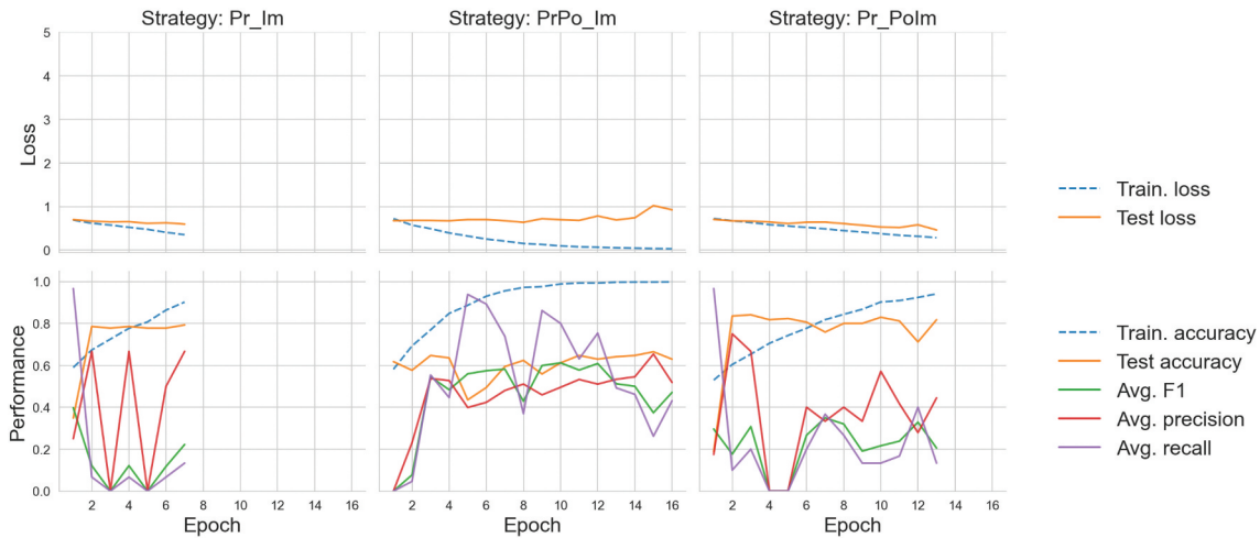
Figure 4. Model performance across three classification strategies for a single training instance in each case. All weighted average metrics were computed on the test set.
